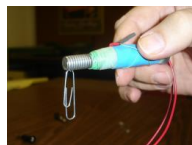
Build an Electromagnet
